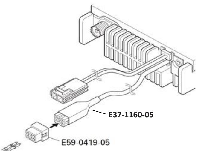
(KAP-2) Which Includes Option Cable E37-1160-05 & Connector E59-0419-05 For Receive Audio Output
