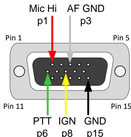
Note: MIC Hi has a 4.7KΩ series resistor
